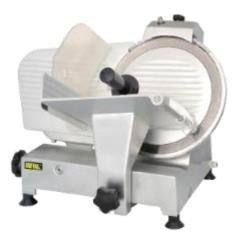
Electric manual meat slicers use a powerful motor to spin a circular blade at high speeds. The user then slides the meat carriage from side to side, accurately cutting the meat to a set thickness. These are sometimes called *gravity slicers* or *self-feeding* slicers as the food carriage is slanted to push the meat against the blade.
